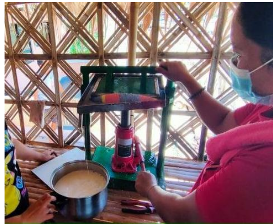
Figure 15. BFA member extracting coconut milk using a mechanical presser
