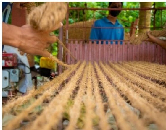
Figure 11. BFA member making the coco coir using loom weaving machine
