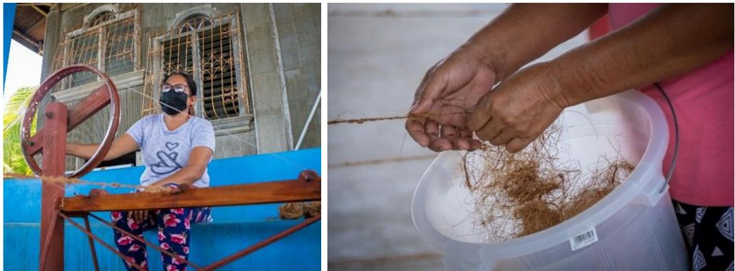
Figure 17. Women members of BFA twining the coco fiber, one working on the spindle to twist the fiber (left) the other feeding out the twined coco coir into the basket.
