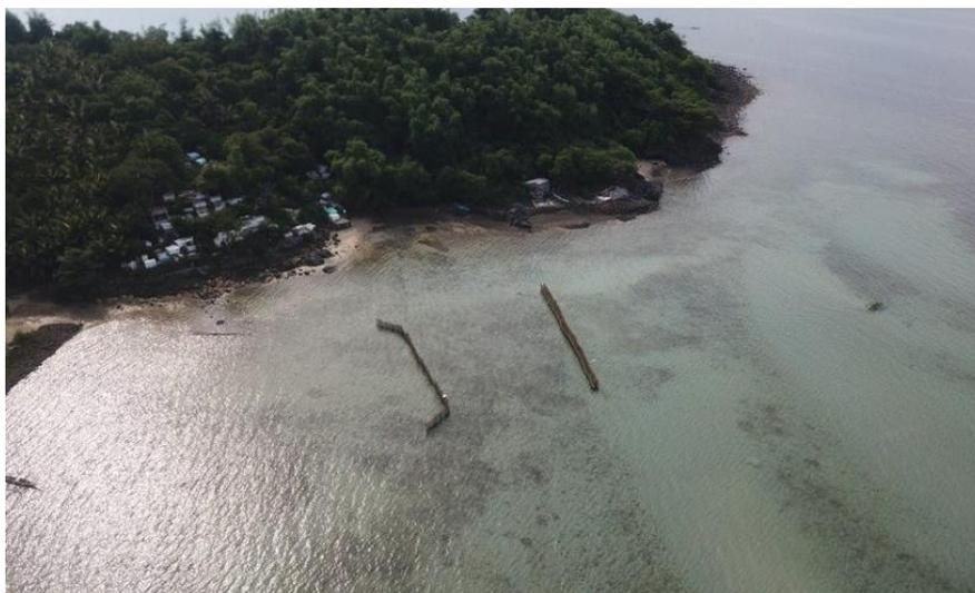
Figure 6. Top view of wave attenuation fence (right) and sediment trapping fence (left).
