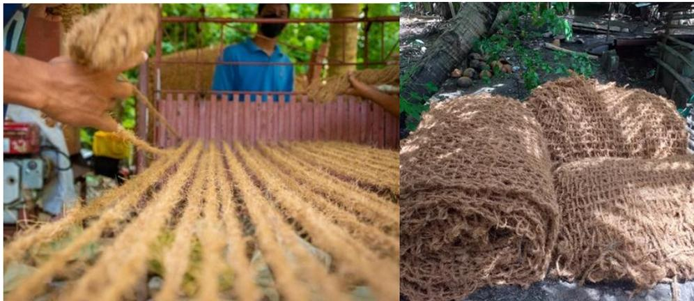
Figure 18. BFA members operating the weaving machine (left) to produce geonets (right) from twined coco coir.
