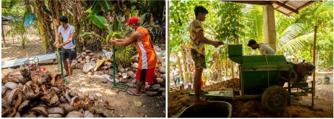
Figure 16. Male BFA members dehusking the coconuts (left) and feeding the husks soaked overnight into the decorticating machine.
