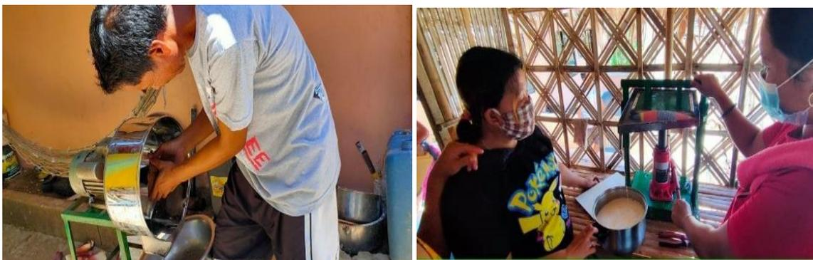
Figure 22. BFA members extracting coconut meat using the electric grater (left) and coconut milk using mechanical presser (right).
