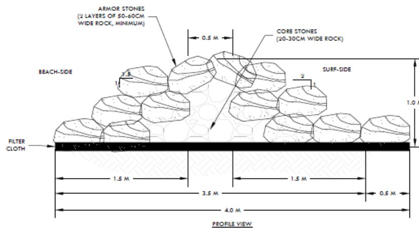
Figure 7. Details of the design of the semi-permeable living breakwater in Loong.
