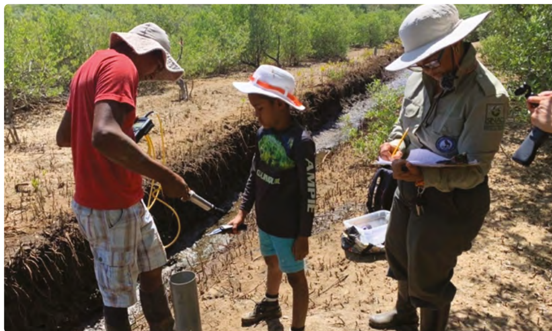
Determination of salinity, redox potential, pH and pore water temperature in an Avicennia germinans forest at a site in Central America. © C. Agraz Hernández
