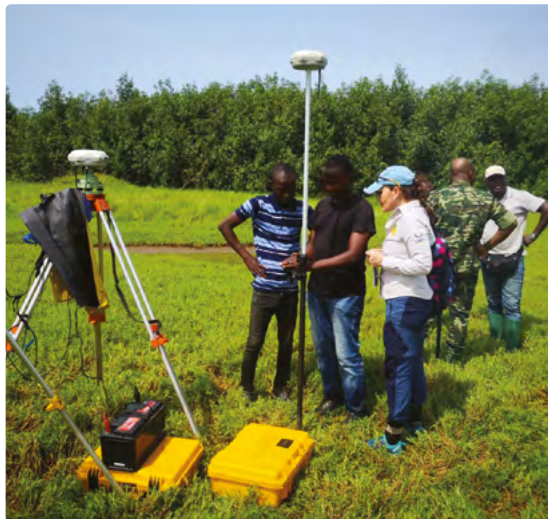
Figure 19. Determining topographic level using RTK methodology in Benin (photo above) and distribution microtopography of a degraded mangrove forest at a site in Cuajiniquil, Costa Rica, 2018 (photo page p47).
