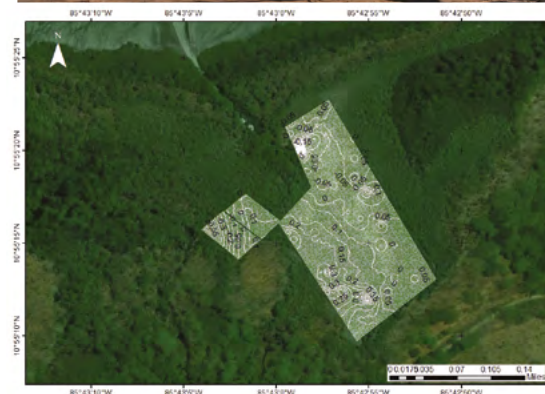
Figure 14. Map of the microtopography of the area to be restored using the RTK method (Cuajiniquil)
